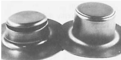
14.2. Drawing failures by necking at the bottom of the cup wall. From D. J. Meuleman, PhD thesis, University of Michigan (1980).
