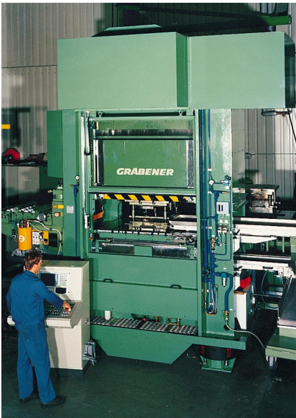
◀ Fig. 4.4.9 Universal press with modified top drive (nominal press force 8,000 kN)
