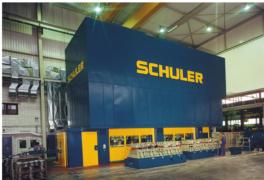
▲ Fig. 4.4.23 Mechanical transfer press for the production of wheel hubs nominal press force: 42,000 kN; number of stations: 11; feed pitch: 700 mm; slides: 3; strokes per minute: 10-28
