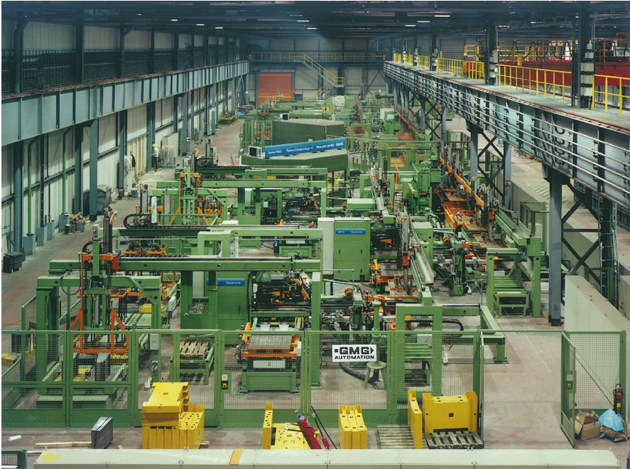
▲ Fig. 4.6.25 Blank welding line with continuous part handling system for the manufacture of welded side members (cf. Fig. 4.4.12)
