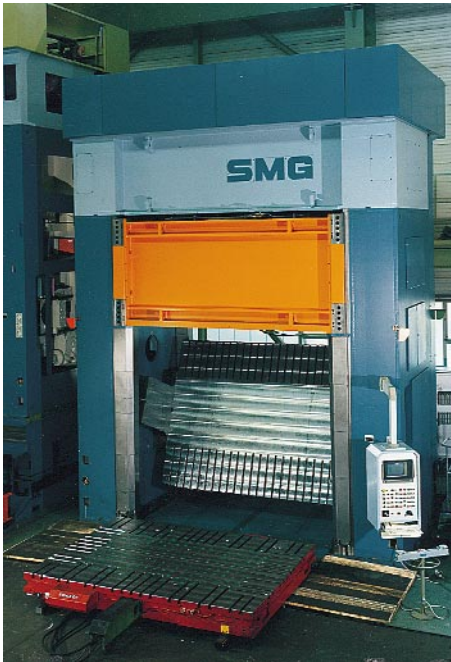
◀ Fig. 4.1.21 Rotating the slide of a hydraulic try-out press
