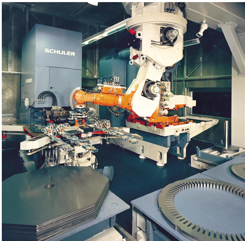
▲ Fig. 4.6.17 Flexible automatic notching machine with robot and pallet magazine (nominal press force 250 kN)
