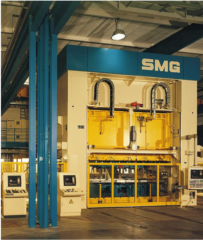
◀ Fig. 4.4.25 Hydraulic transfer press: nominal press force: 42,000 kN; number of stations: 11; feed pitch: 700 mm; slides: 3; strokes per minute: 10-28
