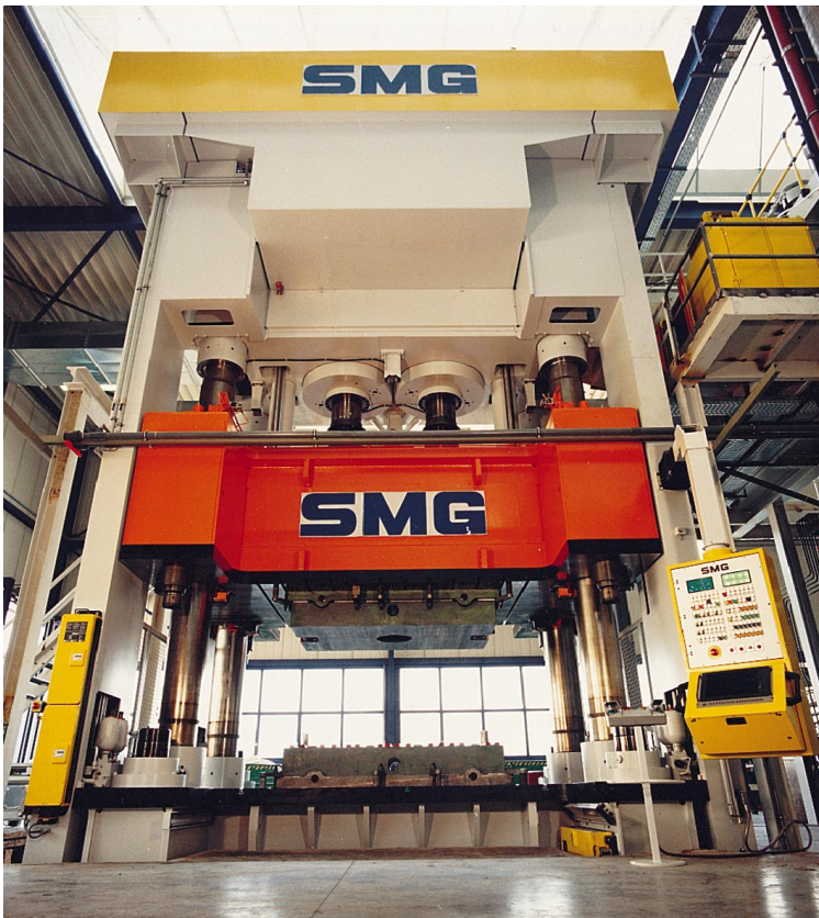
▲ Fig. 4.4.40 Hydraulic plastic press for SMC and FRTP parts nominal press force: 18,000 kN; maximum stroke: 1,300 mm
