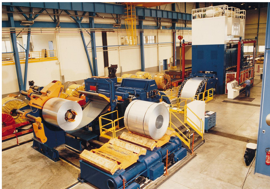
▲ Fig. 4.3.1 Coil line for direct feed of stock material into the press
