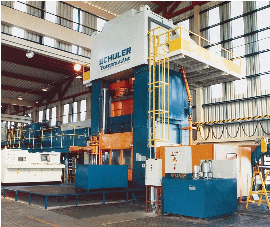
▲ Fig. 6.8.5 Warm forming line comprising a multiple-station press with eccentric drive (nominal press force 20,000 kN, induction furnace, transfer feed and die change support)
