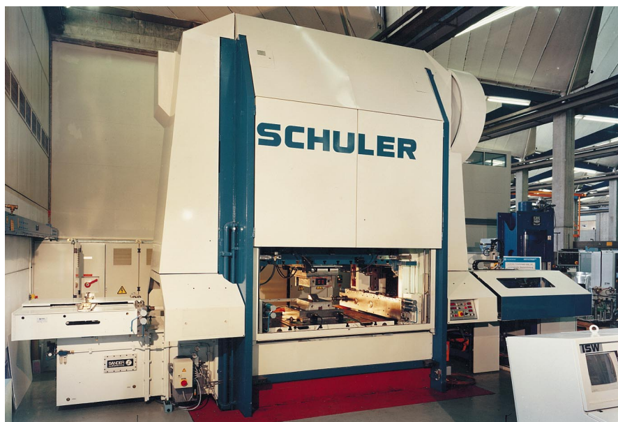
▲ Fig. 4.4.5 Hybrid press (nominal press force 3,150 kN)
