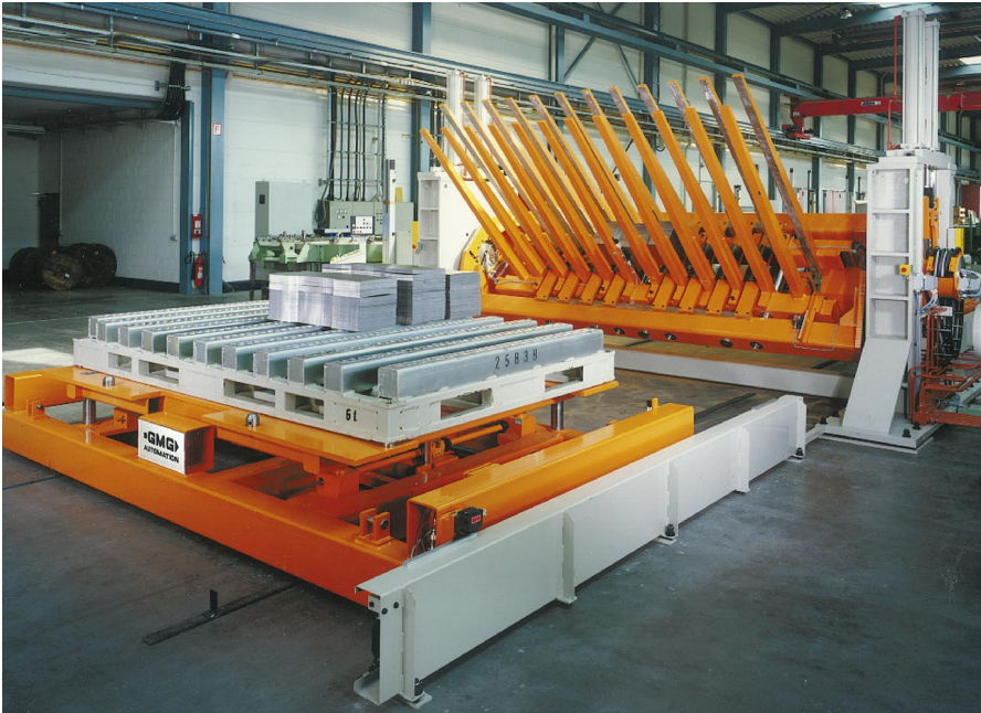
▲ Fig. 4.4.18 Blank turning device for multiple stacks
