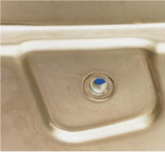
◀ Fig. 4.1.5 A pressed part with an integrated punched nut
