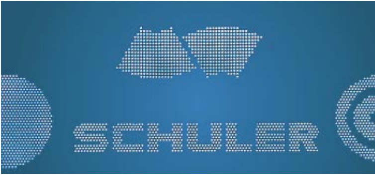
▲ Fig. 4.6.32 Examples of hole patterns produced on a strip perforating press
