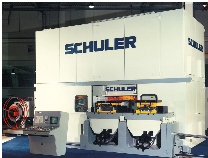
▲ Fig. 4.6.6 Blanking line with 1,250 kN high-speed press and die changing cart for automatic die change (long version)
