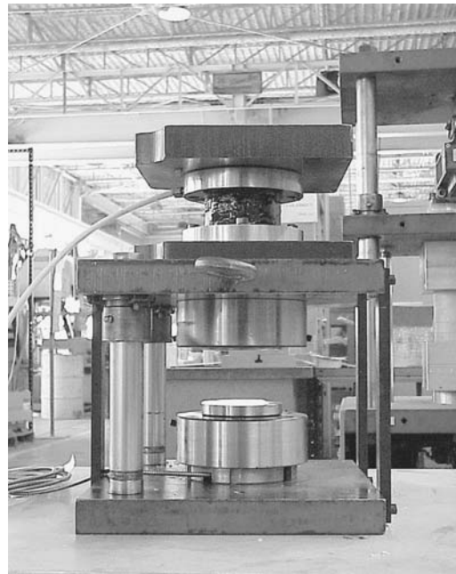
Fig. 4.5 Compression test tooling. [Dixit et al., 2002]
