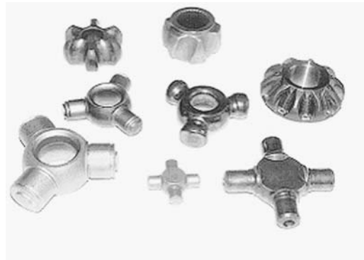
Fig. 23.1 Examples of net shape forged parts [Meidert et al., 2000]
